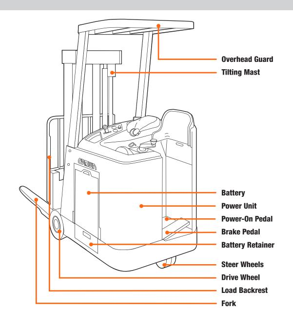
9 Lift Truck Parts Lift Truck Parts 10
