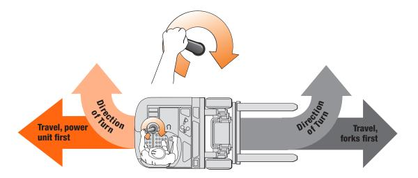
**PRONT DIRECTIONAL STEERING (Sometimes called Forward Steering.)**Shows direction truck will turn when steering handle is turned clockwise.
